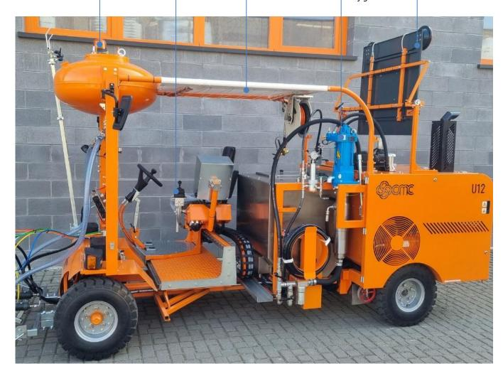
**Seats** and console unit **sliding** (left/right) up to above marking unit *only with hydraulic steering*
