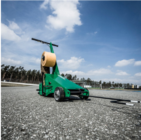
Foil laying technology
