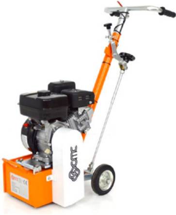
Marker cutters with 20 cm working width
