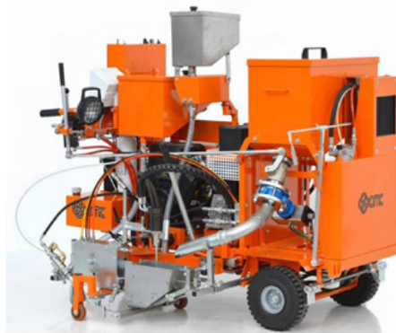
Cold plastic machines with hydraulic drive
