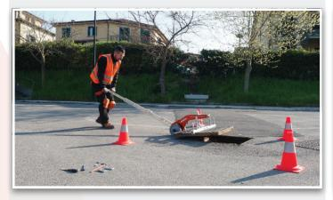
The Hook System extends the Valifter's lifting system possibilities, allowing them the mechanical anchoring on the manhole covers.
