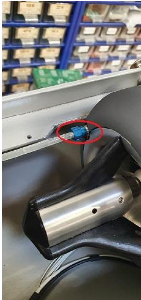
Figure 33 - Secured fuel connection
