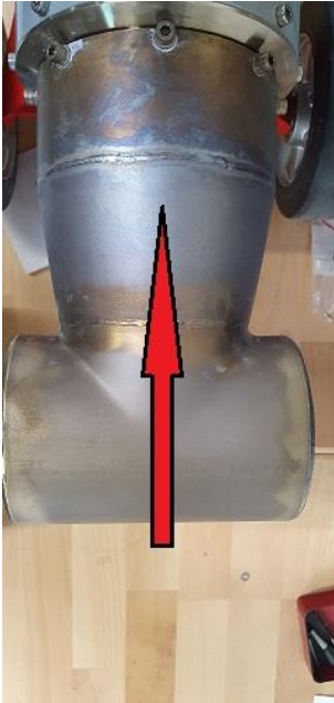
Figure 29 - Turbine module insertion
