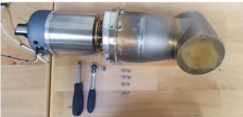
Figure 28 - Turbine module installation tools
