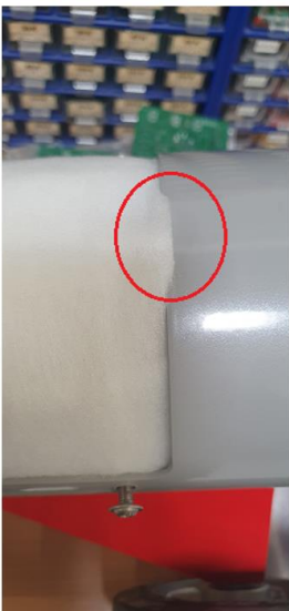
Figure 40 - Wrong vs Right installation of the air filter
