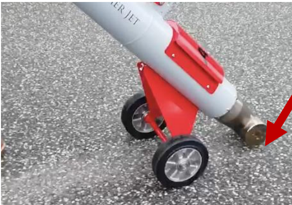
Figure 6 – Nozzle opening position for optimal drying speed.
