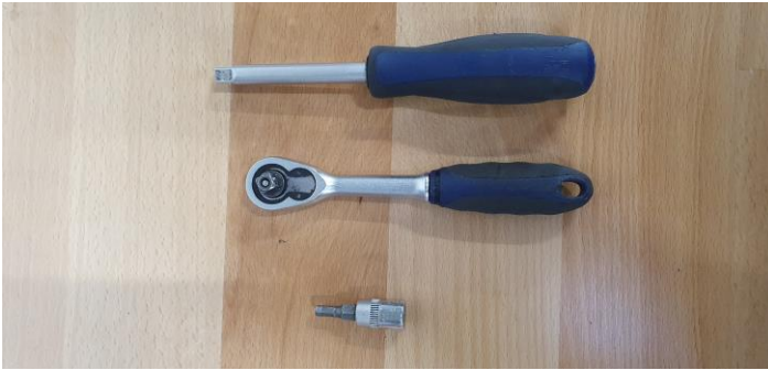
Figure 23 - Tools for dismantling the turbine module
