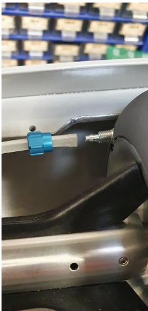
Figure 32 - Loose fuel connection
