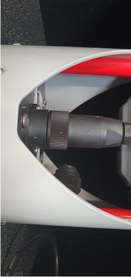
Figure 36 - Secured charging connection
