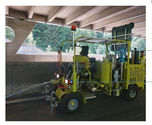
Airless piston pump, airless configuration
