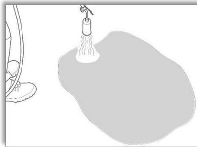
2. If the asphalt is aged it is an advantage to treat the surface with a sealer/ primer MeltMark® PRIMER (see separate description/ datasheet). Mark the area where the marking will be positioned with a chalk. Use a roller or brush. The **primer must completely dry** before continuing to the next step. **Do not position the marking until the primer is completely dried.**
