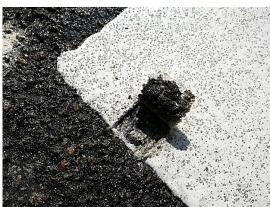
**5.** The material cools normally within 5-10 minutes. When the material has completely cooled an adhesion test can be performed with a hammer and chisel. Good adhesion is achieved when parts of the asphalt surface has adhered to the back side of the marking (see picture above). To speed up the cooling during hot days sprinkle with some water. Remove surplus/ non-attached glass beads after application is completed.
