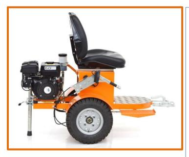
HMC is a hydraulic motorized chariot, to move the line stripers L40-PRO, AR30-PRO, A30PRO-P, AR30PRO-2C and AR30PRO-P-2C, useful to increase productivity and reduce operator fatigue
