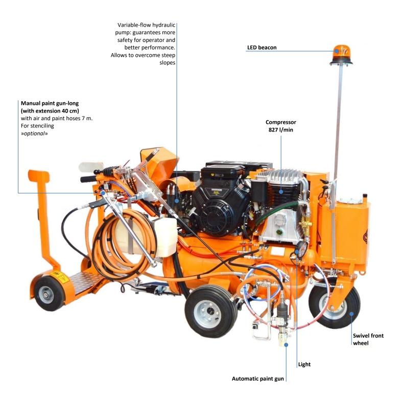
Automatic paint gun can be mounted on fixed support with adjustable height (standard), on one-disc pneumatic support (optional), on marking discs (optional).
